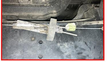
Install the rear wheels. Lower the vehicle to the ground. Torque the lug nuts to the wheel manufacturers specs. Torque the upper and lower rear shock hardware and the U-bolt nuts to 90 ft-lbs. Check to make sure that your e-brake functions properly.
