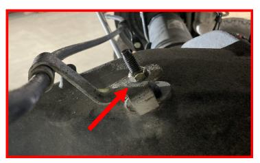
Install the provided e-brake bracket extension to the factory bracket with the provided hardware. Torque to 15 ft-lbs.
