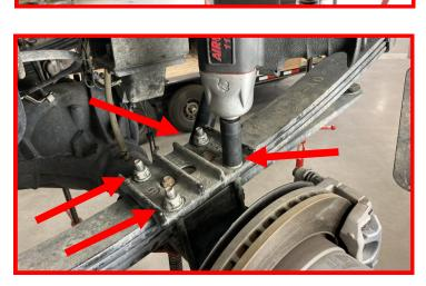
Lower the axle carefully to be able to install the included taper block.
