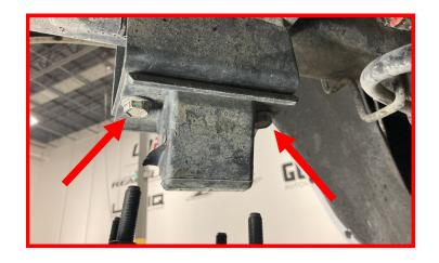
Install the bump stop extension onto the frame using factory hardware.
