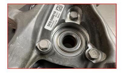
Remove hub assembly from factory knuckle.
