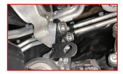
Remove the (3) driver side rear differential mounting hardware. Retain the factory hardware.
