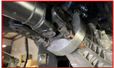
NOTE: Some models you will need to trim the plastic bracket on the side of the transmission due to contact with the driveshaft.
