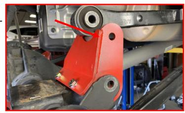
Install the upper control arm crush sleeve between the upper control arm bracket and the control arm axle mount.
