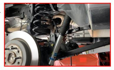
Install the rear bump stop extension on the axle pad.
