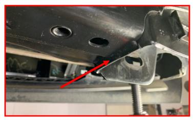
Install front crossmember using the supplied cam block off plates, M18 bolts, washers, and nuts.
