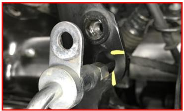
Remove brake line from factory mounting area.
