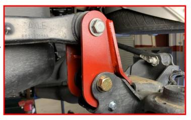
Remove the frame side track bar mounting bolt.
