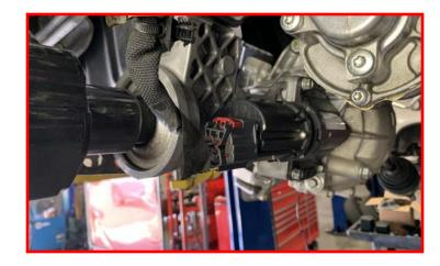
Install the top harness retaining clip into the shift solenoid harness bracket.
