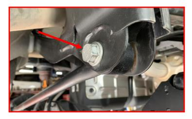
Install track bar bracket using the 14mm x 70mm bolt, washers, and c-lock nut in the track bars original location. Do not tighten at this time.
