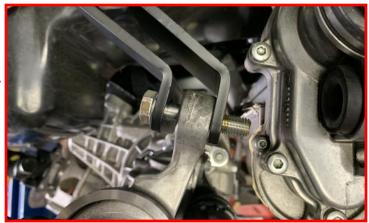
Install shift solenoid harness bracket onto the (2) M12 bolts used to mount the passenger side differential in the previous step. Install the supplied M12 locking nuts and washers.
