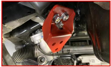
Raise differential into place. Be sure to use a helper to aid in the installation process. With the differential in place, install the provided M12 x 60mm bolt, washers and nut through the driver side inner differential drop bracket, the diff drop spacer, the differential housing, then the driver side outer differential drop bracket.
