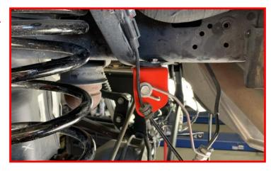
While gently pulling down on the brake line install the factory brake line bracket onto the rear track bar bracket using the factory hardware and supplied M8 nut and washer.
