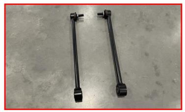
Install the sway bar end links using factory hardware. Do not tighten at this time.
