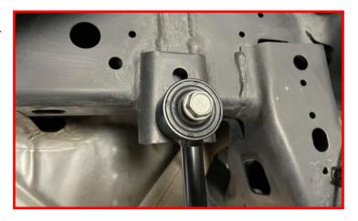
Install the sway bar end links using the supplied M12-1.25mm serrated flange nut. Do not tighten at this time.
