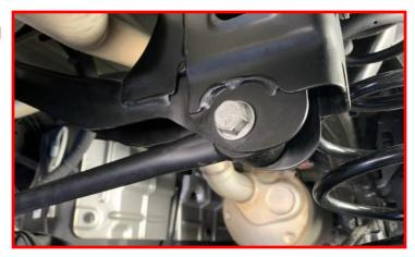
Lower the axle down enough to remove the springs and rubber isolator.
