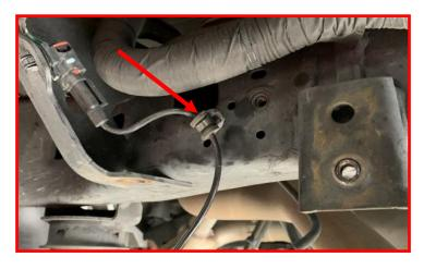
Remove the harness retaining clip from the top of the rear differential.
