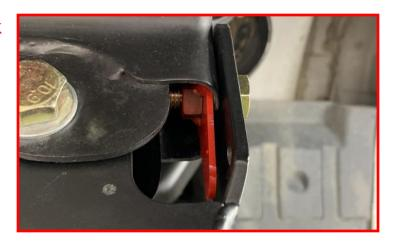
Install the track bar into the track bar bracket using the factory hardware. Do not tighten at this time.
