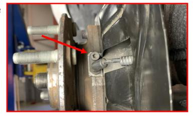
Remove rubber isolator from the ABS bracket on the inside of the knuckle.
