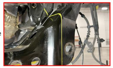
Install the driver side differential drops onto driver differential mounting point using the supplied M14 x 100mm bolt and washer. Do not install the back side M14 washer and nut at this time.
