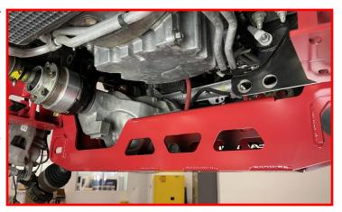
Install the rear diff mount into the rear crossmember using the supplied M14 x 100mm bolt, washers and lock nut.
