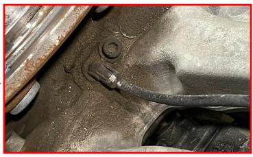
Remove the CV shaft retainer nut.
