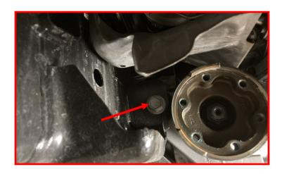
Remove the passenger side diff mounting bolt.
