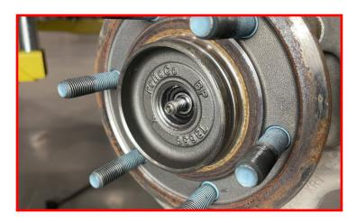
Remove the (4) bolts that attach the EI-WE to the knuckle and pull both axle and the EIWE out of the factory knuckle.
