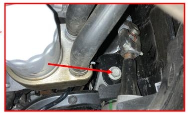
Remove the rear diff mounting bolt.
