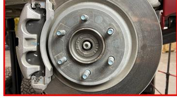
Install the CV shaft retainer nut dust cover.
