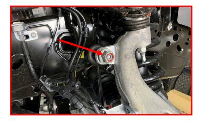
Remove the tie rod end on the knuckle.
