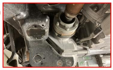
Remove the passengers side CV by striking the shaft with a hammer to dislodge it from the splines.
