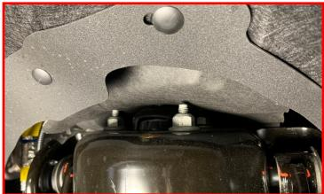
Remove the lower strut nuts.
