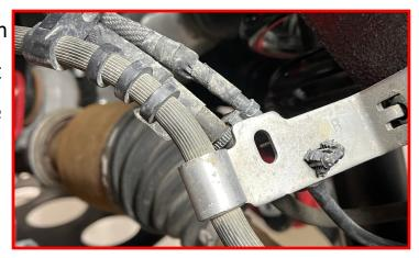
Install vacuum line onto brake line bracket.
