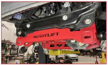
Install the driveshaft spacer and driveshaft in the same orientation with the marks previously made using the 10mm x 100mm Allen head bolts and a drop of thread locker to all bolts.
