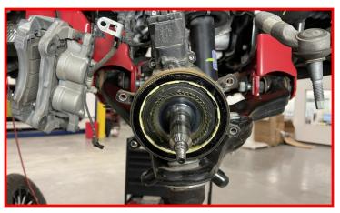
Install the knuckle onto the lower ball joints using factory ball joint nut. Run the nut tight at this time.
