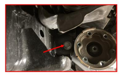
Remove the passenger side diff mounting bolt.
