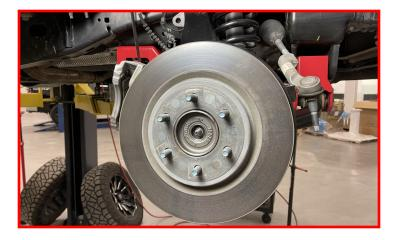
Install the brake caliper assembly to rotor and knuckle using the factory hardware and thread locker.
