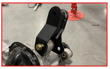
Install the passenger side differential drops onto passenger differential mounting point using the supplied M14 x 100mm bolt and washer. Do not install the backside M14 washer and nut at this time.
