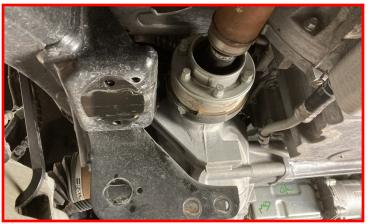
Remove the passengers side CV by striking the shaft with a hammer to dislodge it from the splines.
