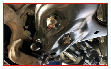
Remove the upper control arm ball joint nut.
