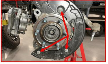
Remove the ABS sensor from the hub assembly.
