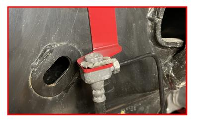
Install the factory brake line bracket to knuckle using the supplied  $M8 \times 16$ mm bolt, and washer
