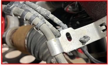
Install vacuum line onto brake line bracket.
