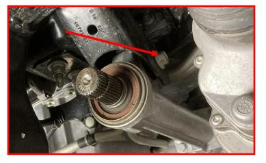
Disconnect the differential breather hose from the differential housing.
