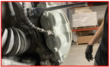
Carefully remove the brake rotor.
