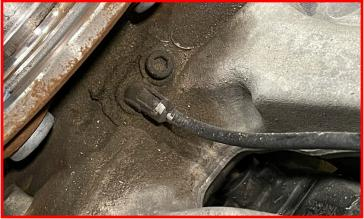
Remove the CV shaft retainer nut.
