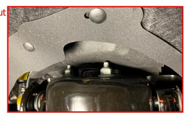
Remove the lower strut nuts.
