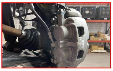
Fasten the CV shaft to the hub with the factory nut.
