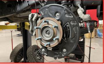
Carefully install the brake rotor onto the hub assembly.
