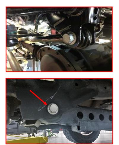
Loosen the rear radius arm bolt.
