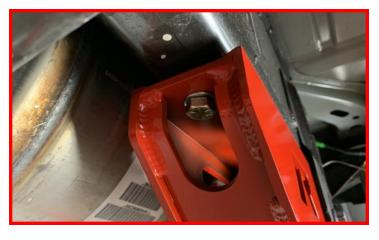
Bend the wires to align the tab nut with the front mounting holes in the bracket and frame. Install the provided 1/2" bolts and washers.
