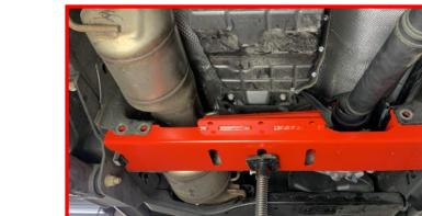
Using the factory transmission crossmember hardware, install the driver side bolts from front to rear.
