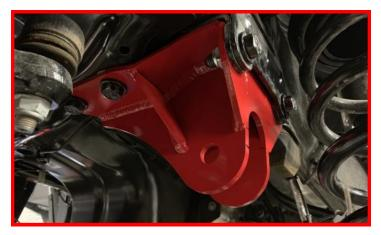
Install track bar using factory hardware.
