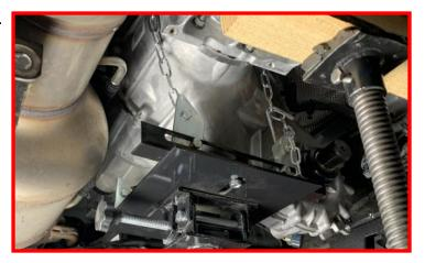
Remove the (8) transfer case mounting nuts.
