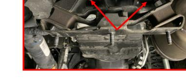
The remaining (2) bolts are located at the front of the mount. Remove the (2) bolts and remove the mount.
