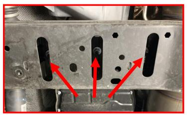
Remove the (3) transmission mounting nuts.
