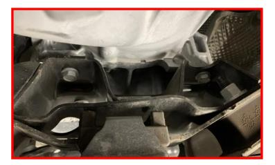
Tighten the transmission mount bolts.
