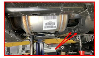
Lower jack and install the (2) Diesel Exhaust Fluid (DEF) tank crossmember exhaust hanger bolts.
