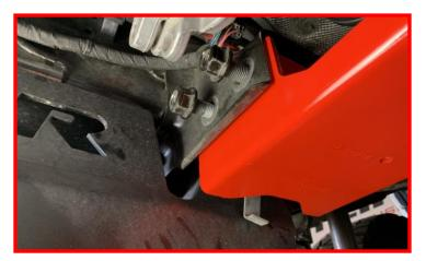
Using the (2) provided hardware bolts install the passenger side bolts from front to rear. This will aid in removal if service needs to be performed.
