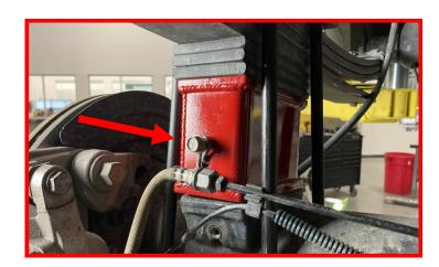
Install the e-brake bracket on top of the differential stud using the provided hardware to secure it down.
