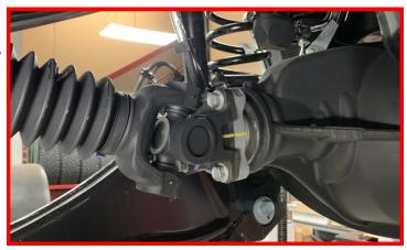
Rotate the axle to release radius arms from the mounting locations.
