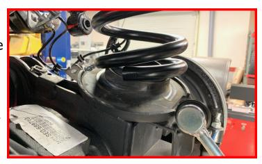
Passenger side ends up with end of the weld on the lower cup to axle/track bar mount.
