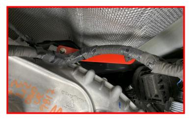
Install the transfer case shift solenoid connector.
