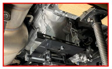
Remove the (8) transfer case mounting nuts.
