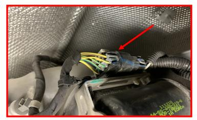
Remove the transfer case harness retaining clip on the rear of the transfer case.
