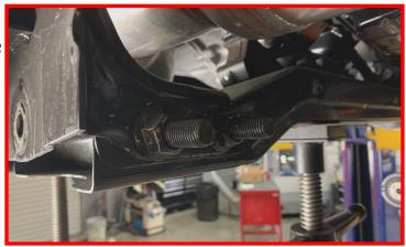
Note: Vehicles that are equipped with optional diesel engines, It will be necessary to raise the DPF (Diesel Particulate Filter) to remove passenger side transmission crossmember bolts. The following steps will instruct you on how to proceed.
