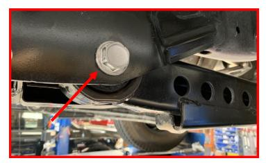
Mark the driveshaft to pinion location. Remove the <u>front driveshaft</u> from the axle. Let hang out of the way.
