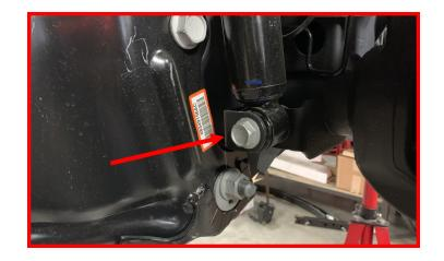
Place a jack under the axle for support. Remove the radius arm bolts.
