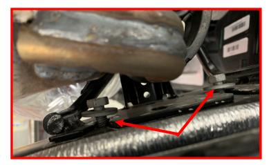
Install the (2) center exhaust hanger mounting bolts.
