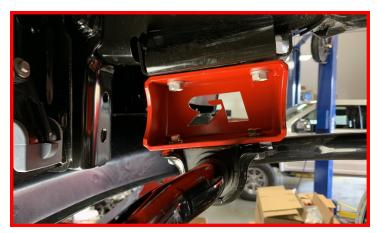
Install provided brake line extensions to the frame brake line brackets using the provided 5/16" hardware. Do not tighten at this time.
