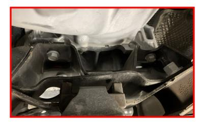
Tighten the transmission mount bolts.
