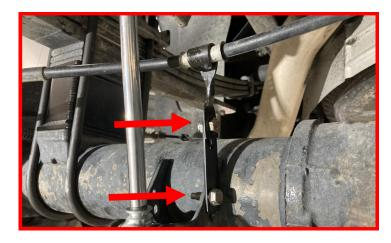
Remove the tree connector holding the top of the axle breather tube and secure it in a lower position using the factory connector and the provided hardware.
