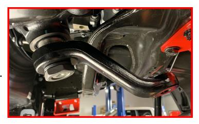
Loosen tie rod end adjuster and rotate tie rod end 180 degrees. Attach tie rod end to pitman arm using factory hardware.
