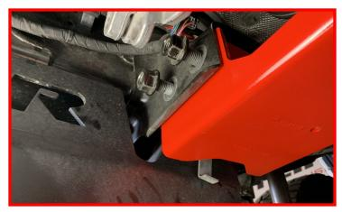
Using the (2) provided hardware bolts install the passenger side bolts from front to rear to avoid hitting the DPF. This will also aid in removal if service needs to be performed.
