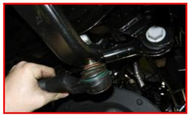
Loosen but do not remove track bar bolt at the axle.
