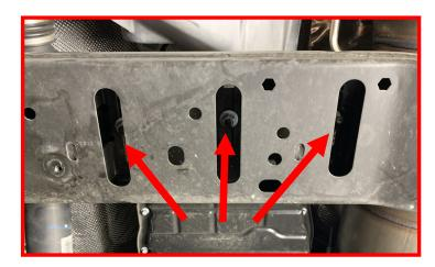
Remove the (3) transmission mounting nuts.
