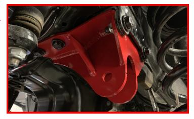
Install track bar using factory hardware.
