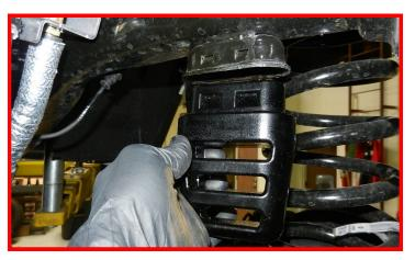
Using an appropriate cutting tool, remove the alignment tab on the coil spring isolator.
