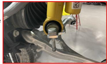
Continue to raise the lower control arm up until you are able to install the supplied M12 Lock nuts and washers.
