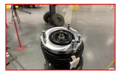
Using the supplied M10 flange nuts, Install the strut assembly into the vehicle in the factory orientation.
