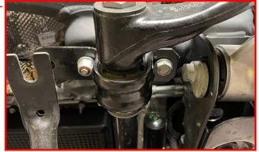
Remove both the driver and passenger rear sway bar retainer cap nuts.
