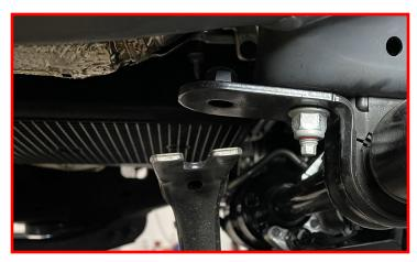
Tighten the (2) forward sway bar skid plate bolts.
