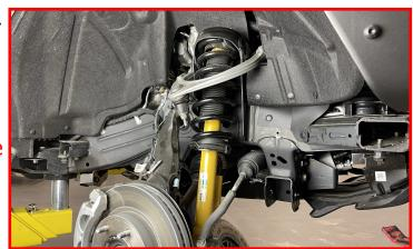
Install the top strut spacer onto the strut assembly.
