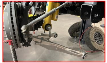
Remove the (3) top strut nuts and carefully remove the strut assembly from the vehicle.
