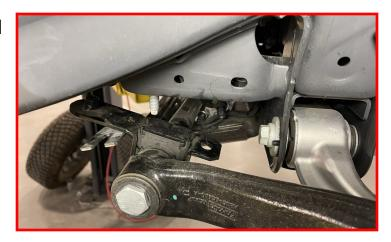
Remove the lower control arm pivots from the frame side pivot pockets.
