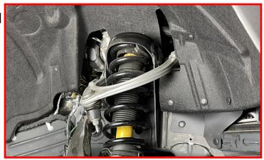
Install the lower strut spacer onto the lower strut studs.
