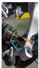
Loosen but do not remove the lower control arm (LCA) hardware at the frame. Lower the LCA while supporting the knuckle and remove the strut from the vehicle. Take care to not over extend or stretch the ABS-rubber brake lines and CV axle. Adjust as necessary.
