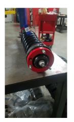
Reinstall the strut into the truck. 1st align the top hat to the strut tower, use three of the supplied flange nuts, hand tighten at this point only.
