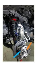
use a hammer to dislodge the axle from the wheel bearing. Use cation with this, don't strike the axle with the hammer. use a center punch and align with the center hole on the axle.
