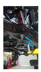
With the upper ball joint nut loose and the tie rod nut removed, strike the ball joint boss with a dead blow hammer to dislodge the taper. Once the taper is dislodged remove the upper ball joint hardware, and separate the UCA and the tie rod from the steering knuckle. Allow the steering knuckle to lean out, for clearance. Take care to not over extend or stretch the CV axle Adjust as necessary.
