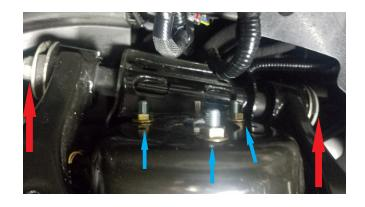
Remove ABS wire from the steering knuckle.
