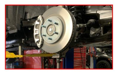
Remove the sway bar end link from the lower control arm.
