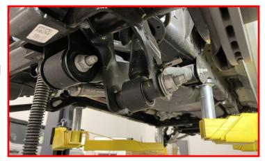
Before installing the top spacer place the strut into a spring compressor. Mark the top hat to spring location.
