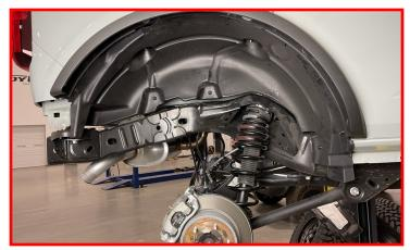
Prior to installing wheels, complete all installation steps on the opposite side. Install the wheels and lower the vehicle to the ground. Torque the lug nuts to the wheel manufacturers specs. Jounce the vehicle to settle the suspension to the new ride height.
