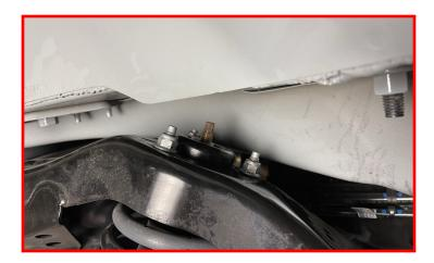
Using an appropriate jack, support the axle.
