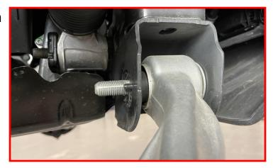
With the lower control arm pivots removed from the frame pockets, Swing the lower control arm down while removing the lower strut studs from the control arm.
