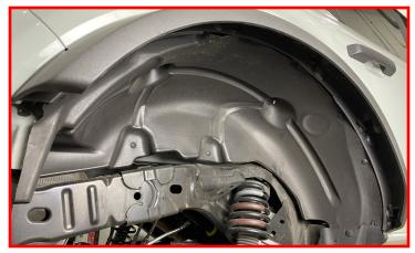
Remove the rear fender liners.
