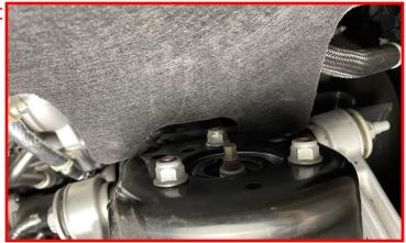
Remove the lower strut nuts.
