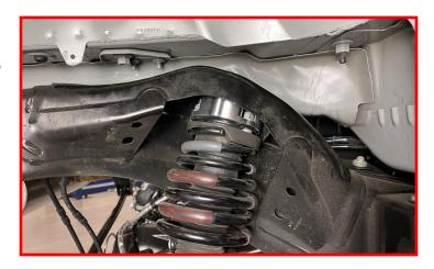
Raise the axle into place and install the lower strut bolts.
