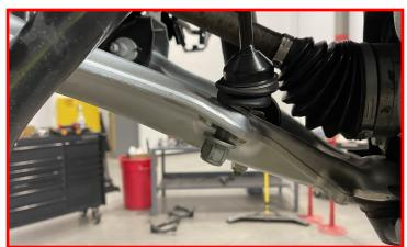
Raise the sway bar back into the factory orientation on the frame.
