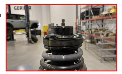
Install the top strut spacer (68-21200RSS) onto the rear strut assembly using the factory nuts.
