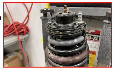
With the rear strut assembly removed from the vehicle, remove the locating pin from the top hat using pilers or similar tool.
