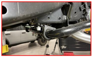
Install the driver and passenger forward sway bar retainer cap bolt.
