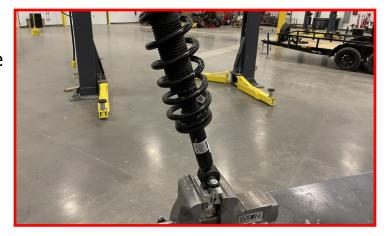
Install the top strut spacer (68-21200FSS) onto the strut assembly using the factory nuts.
