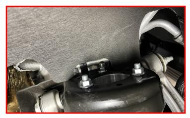
Install the sway bar back into the vehicle in the factory orientation.
