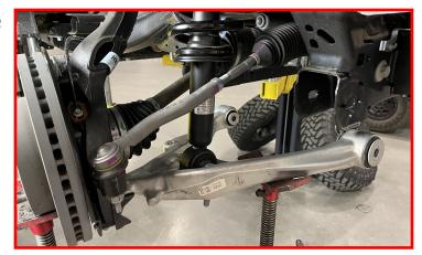
Continue to raise the lower control arm up until you are able to install the factory mounting hardware.
