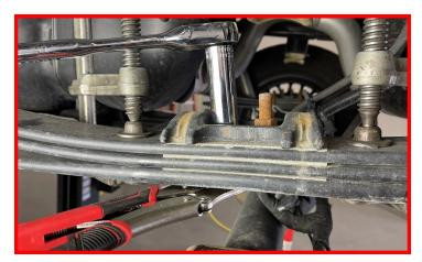
Remove the factory u-bolt retainer plate.
