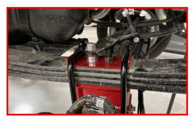
NOTE: IF VEHICLE IS EQUIPPED WITH CCD WITH LOAD SENSING (EXAMPLE OF SHOCK PICTURED) DO NOT INSTALL SUPPLIED SHOCK EXTENSION.
