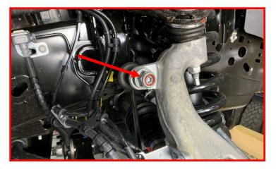
Remove the tie rod end on the knuckle.
