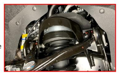
Install the ball joint boot spacer between the bottom of the boot and the top of the knuckle and raise the knuckle high enough to install the ball joint into the knuckle.
