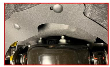
Remove the lower strut nuts. Retain the factory mounting hardware.
