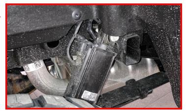
Install the shock extension using the provided M12 bolts, washers, and nuts to the top of the factory shock.
