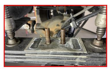
Install the supplied u-bolt retainer plate, Using the factory center pins.
