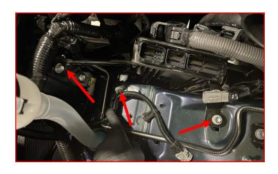
Plug the right most plug into the accumulator and lock it in place by closing the handle to the left.
