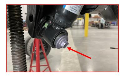
Remove the upper shock nut and bushing.
