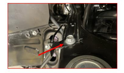
Remove the brake line from the bracket on the chassis.
