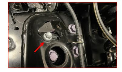
Using factory hardware, install the ReadyLift brake line bracket.
