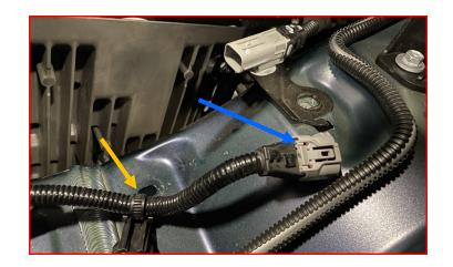
Release the leftmost accumulator plug by pressing in the tab and pulling the handle to the rear of the vehicle.
