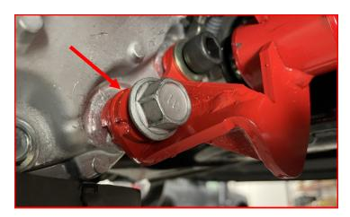
Attach the ReadyLIFT passenger side differential drop bracket to the chassis using factory hardware.
