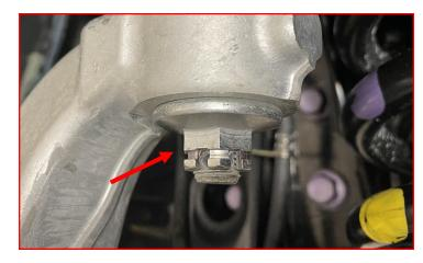
Use the appropriate tool to release the taper on the upper ball joint.
