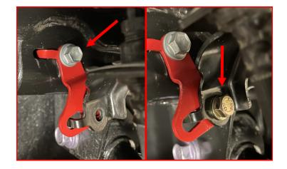
Install the bracket (one on each side) holding the brake line to the axle using factory hardware.
