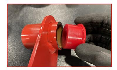
Press the supplied crush sleeve into the bushings until it is flush with the bushing.
