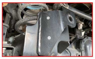
Paint the cut surface to prevent any corrosion.
