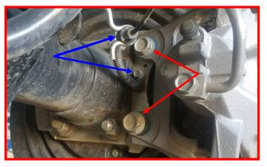
Remove the rear lower shock hardware from the axle mount. Retain the factory hardware
