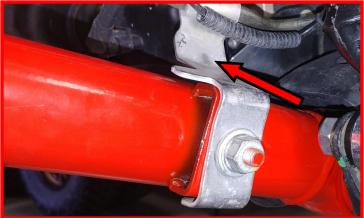
Install the electrical connector that was previously cut to the lower hole in the frame rail. The rest of the harness will hang.
