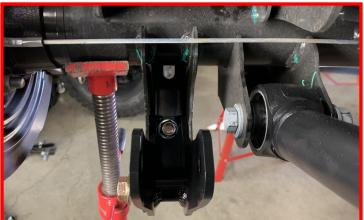
Tighten and torque the M12 hardware to 65 ft-lbs.
