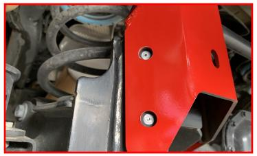
Remove the track bar relocation bracket from the factory axle mount.
