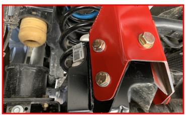
Tighten the U-bolt hardware.
