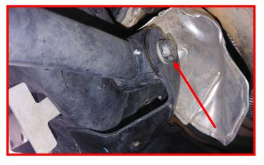
Loosen but do not remove the front upper control arm bolts at the axle.
