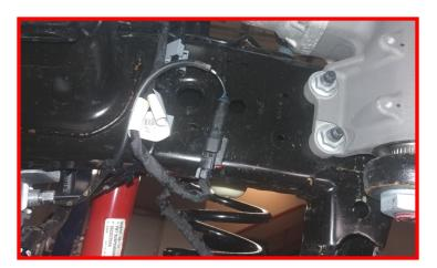
Install the front drive shaft making sure to line up the previous mark using a drop of thread locker and factory hardware. Torque to 40 ft-lbs.
