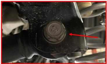
Use caution do not over extend brake lines or wire harnesses. Lower the axle enough to remove the springs. Discard the factory spring at this time.
