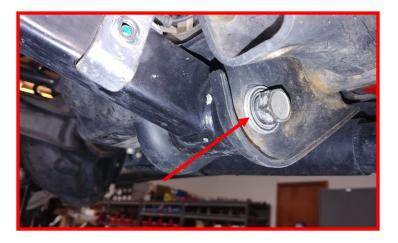
Remove the front lower shock hardware from the axle mount. Retain the factory hardware.
