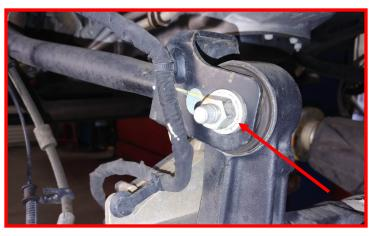
Loosen the front lower control arm hardware at the frame. Do not remove at this time.
