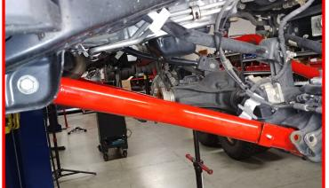
Insert the front bump stop 3/8" x 1.75" Allen bolt into the front bump stop. Insert the front bump stop into the coil spring. Install the coil spring and bump stop at the same time to the frame and axle making sure to clock the spring so that the dead end of the coil sits in the lock on the axle pad. Raise the axle enough to hold the springs in place.
