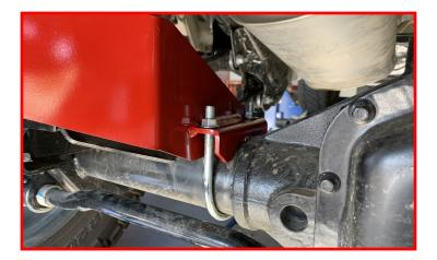
Install the track bar using the factory mounting hardware.
